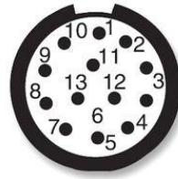
**DC CONNECTORS PIN DESCRIPTION (J3-POWER)****[D38999/20WB98PN AMPHENOL CIRCULAR MIL SPEC CONNECTOR]**
