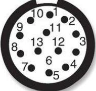
**DC CONNECTORS PIN DESCRIPTION (J3-POWER)****[D38999/20WB98PN AMPHENOL CIRCULAR MIL SPEC CONNECTOR]**
